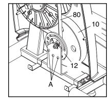
Reattach the left side shield and the left crank arm cover. Then, see step 11 on page 10 and reattach the left pedal leg and the left link arm.
